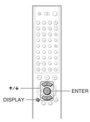
1 Press DISPLAY twice (once for DATA CDs) during playback. The Control Menu appears.
